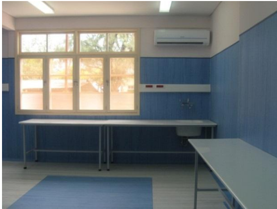
Figure 96: Operable windows: ventilation & daylight, Beira Central Hosp.
