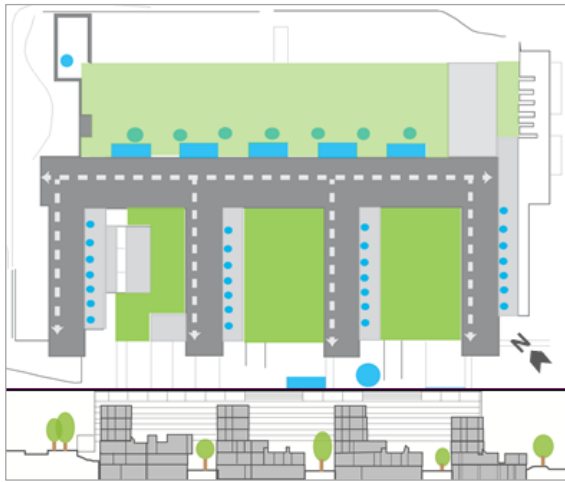
238: Typical Nursing Unit plan and building section, hospital Sant Joan Despi Barcelona
