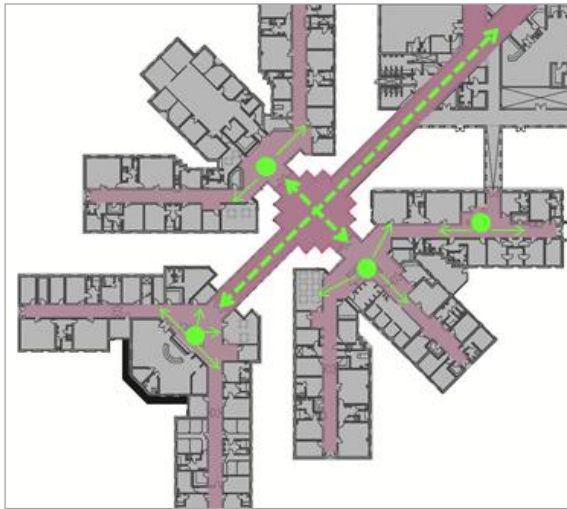
179: Site lines & circulation hierarchy, Vryburg Hospital, SA
